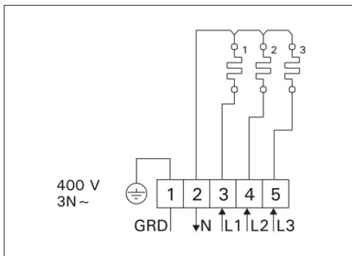
Figure 11. Electrical connections of BC-E heater
