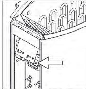
Figure 9. Reset button for overheat protector
