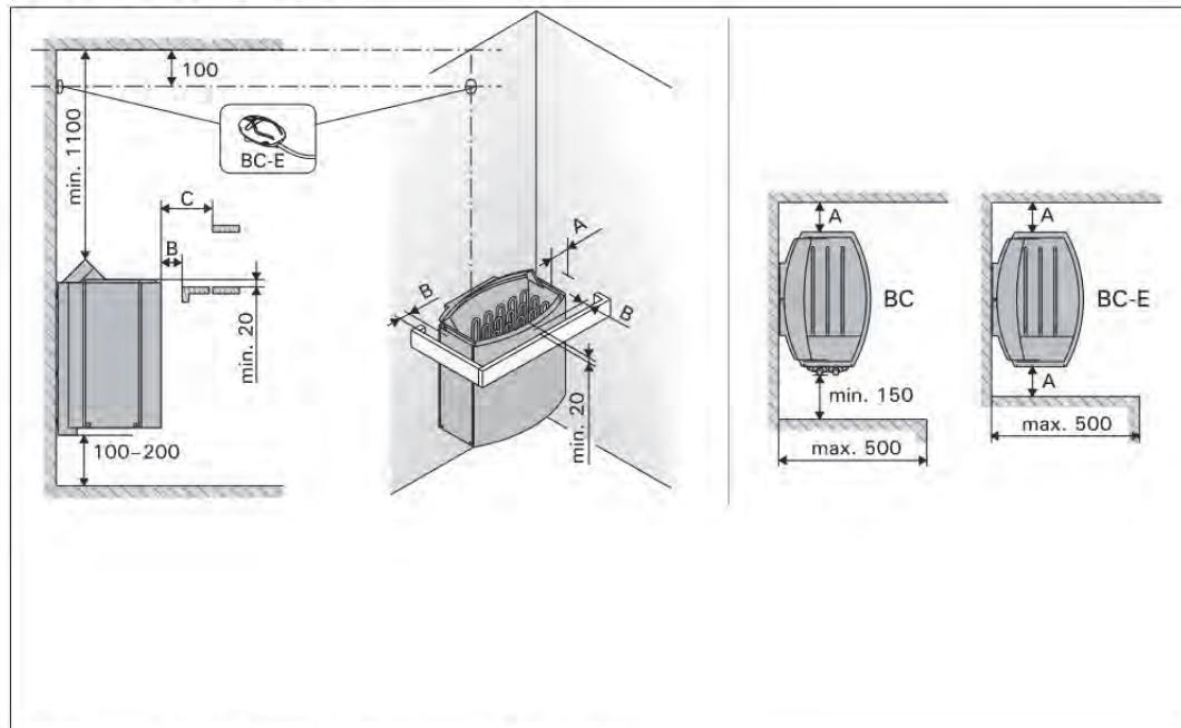
Figure 6. Safety distances (all dimensions in millimeters)
