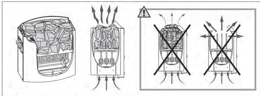
**Figure 1. Piling of the sauna stones**
