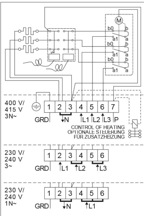
Figure 10. Electrical connections of BC heater
